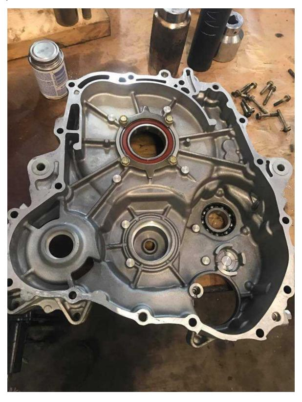
Double checking the oil passage holes to be sure they are clear
