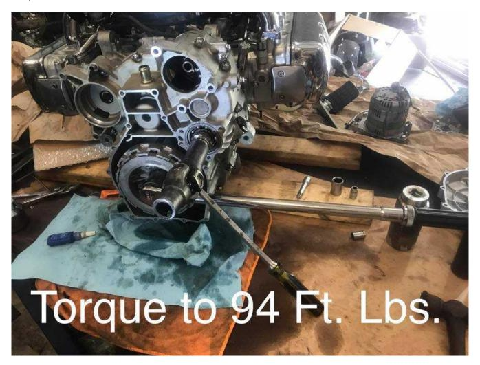
Once it's torqued, stake the nut on both sides to lock it
