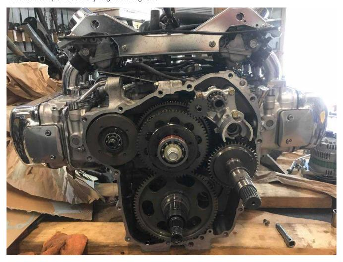
All this work for an \$18 gear that broke due to Hydrolock caused when gas leaks from the OEM petcock from a tear or debris in the diaphragm or Ethanol that has sat deforms the diaphragm cause it to malfunction
