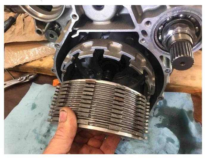
May have to turn the output shaft some to line the splines on the Clutch pack as you are pushing it on
