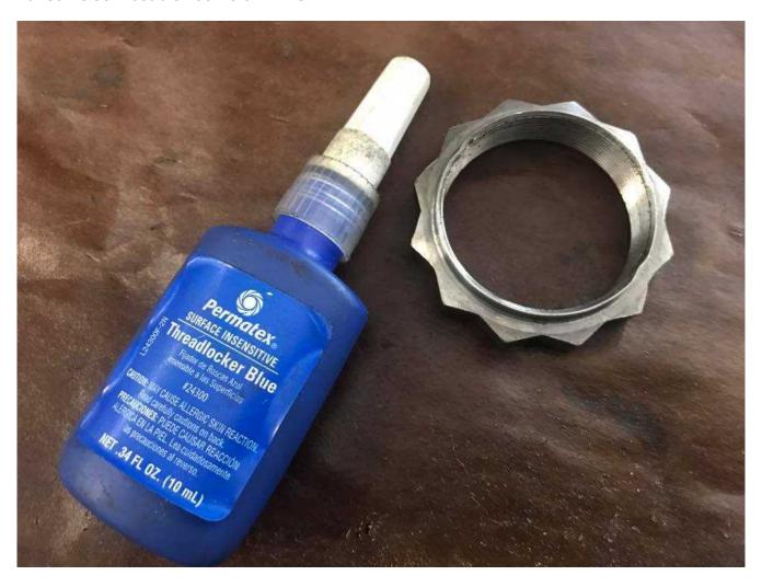
Then torque it down to 137 ft. Lbs. with an 1-13/16" deep socket.
