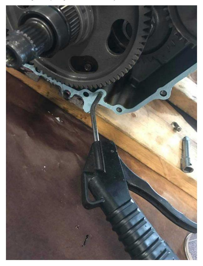
Line up the dowels and shafts through the case holes and push it on
