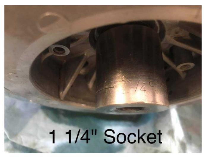
And had to use the u joint and pry bar method on the output shaft to hold it from turning as I torqued it to 94 Ft. Lbs.
