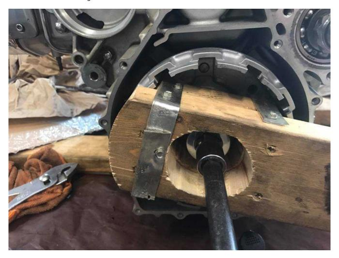
Once the nut is torqued stake the 2 sides to lock it in place
