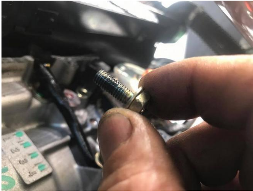
Little blue service removable loctite to keep them from coming loose and losing a tensioner.
