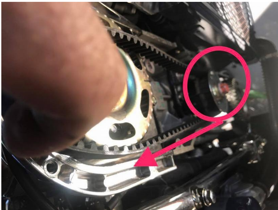
Next put the new right side belt on the outside crankshaft pulley and keep the bottom of this belt from having slack as you work it around onto the camshaft pulley
