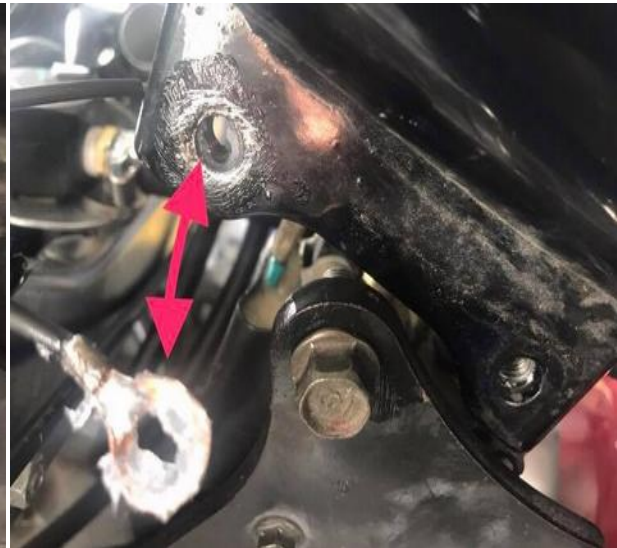
(left) At the top I'm gonna fasten the ground wire in between the frame and bracket so I had to scrape the paint off so it will have a clean connection. It won't be seen it gets covered back up with the outer bracket.
