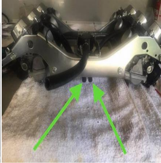
(left) Run the overflow or vent lines out to the carb frame. (right) Poke em in the 2 holes where they go.
