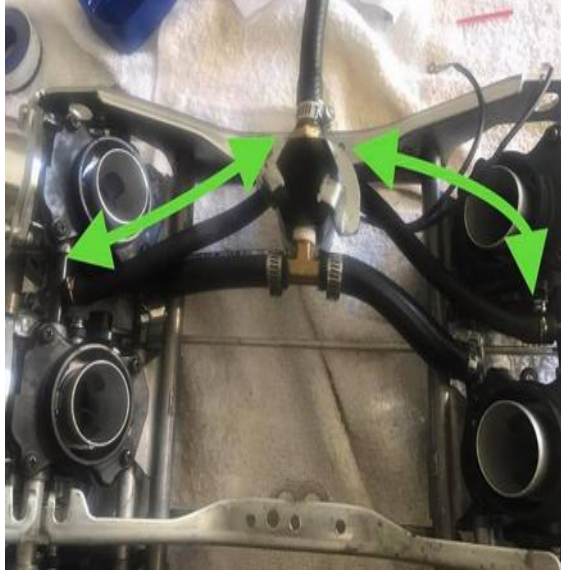
(left) Run the overflow or vent lines out to the carb frame. (right) Poke em in the 2 holes where they go.
