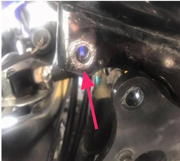
(left) At the top I'm gonna fasten the ground wire in between the frame and bracket so I had to scrape the paint off so it will have a clean connection. It won't be seen it gets covered back up with the outer bracket.
