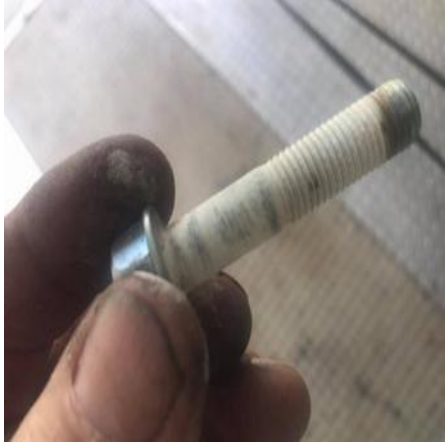
(left) I pulled the bottom bolt out, found it pretty corroded.
