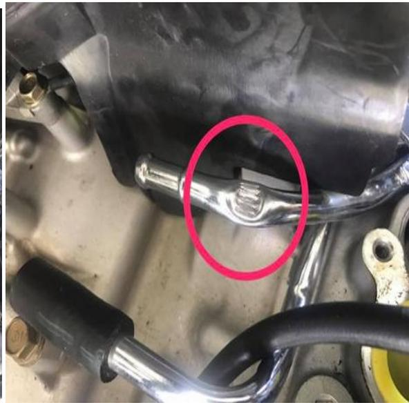
(Left) The front right side tube that comes up from the bottom we are going to crush the tube behind where the intake runner will hide it
