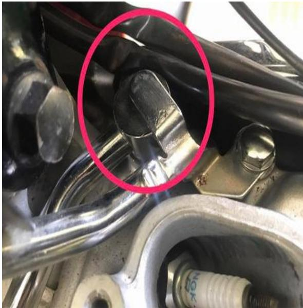
(left) Tab bent down and bolt reinstalled
