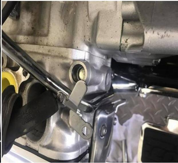
(left) Back left side pull the tube out and drive the next freeze plug in.
