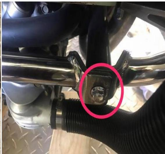
(right) Remove the engine crash bars, I had a picture of all the bolts to remove but am limited to 40 pics per post so had to delete them to make room for other pics. Follow the bars around you'll find the bolts.
