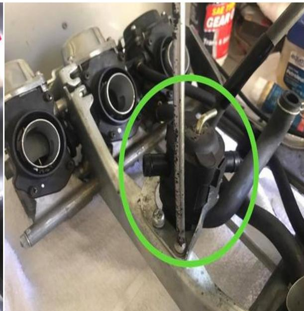
(left) I used a piece of 3/8" fuel line a 12mm bolt and 2 hose clamps.
