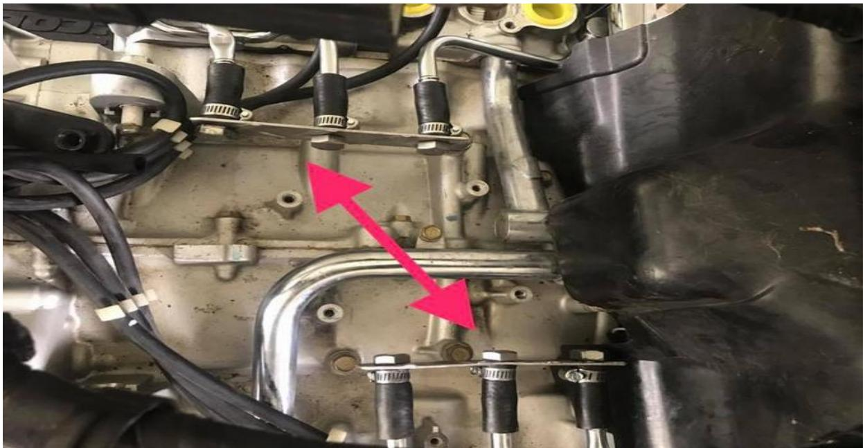
Finished product used the existing rubber tubes that were hooked to the pair valves and stick a bolt thru the plate and into each hose and put a clamp on it. Could probably almost just use the bolts and plates to do the de-smog? One of the guys on here has done it that way and it looks really good.
