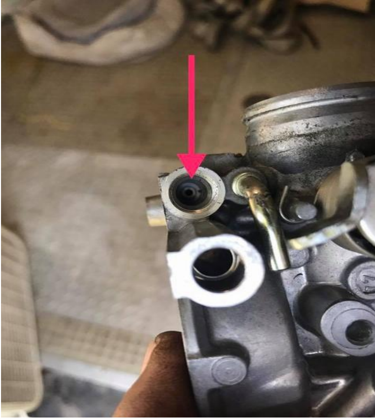
Here's an O ring stuck down in the hole that the picks work great to dig them out
