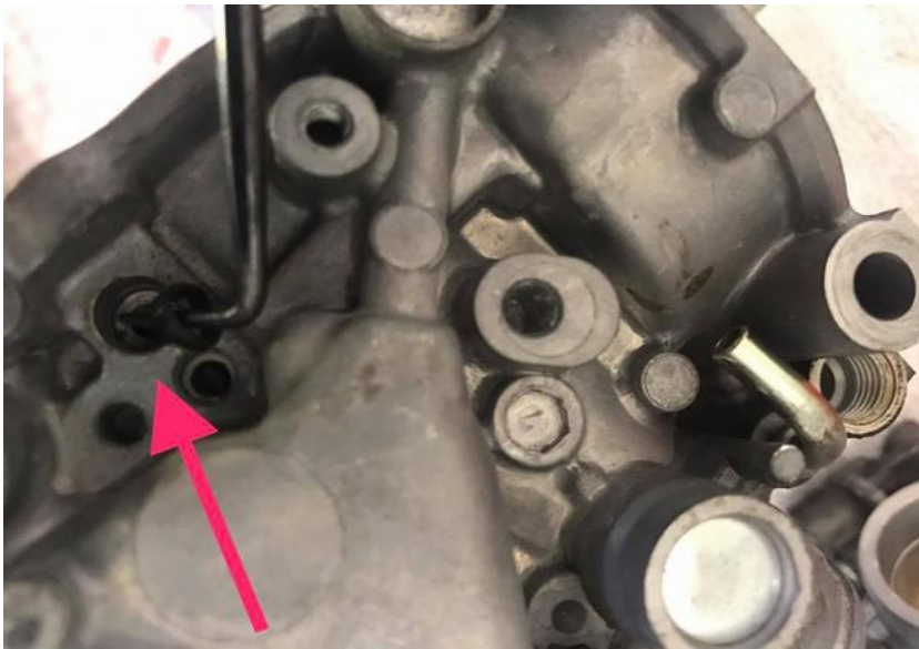
The o rings hide everywhere, look in all the holes to make sure you get them all out
