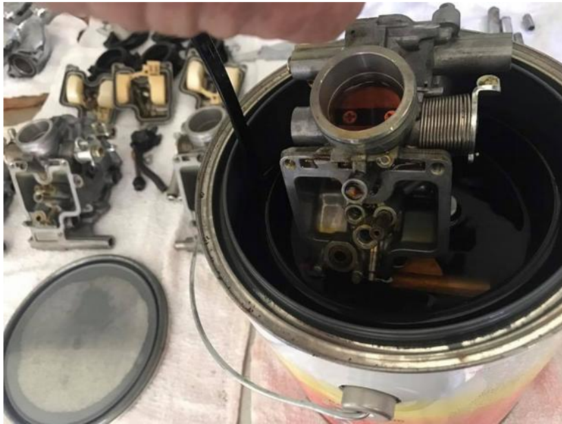
The Berryman cleaner has its own little basket in the can and a whole carb will fit good down in there
