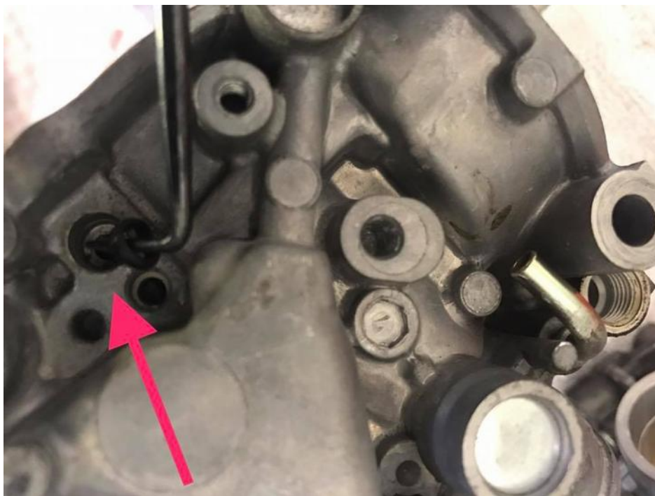
The orings hide everywhere, look in all the holes to make sure you get them all out
