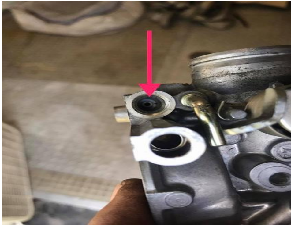
Here's an O ring stuck down in the hole that the picks work great to dig them out
