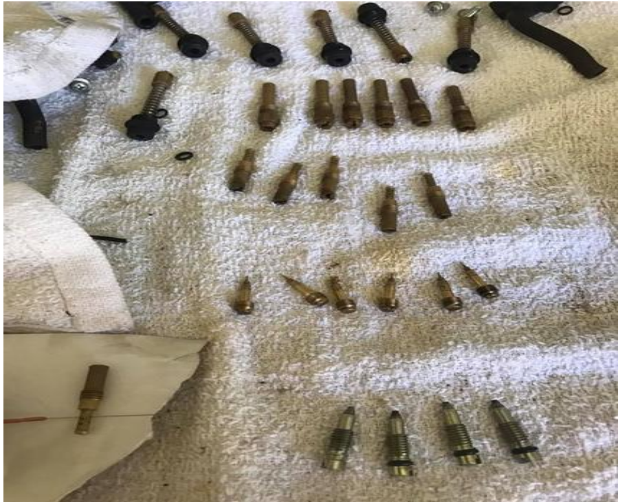
Lots of little jets with lots of little holes, make sure you get them all
