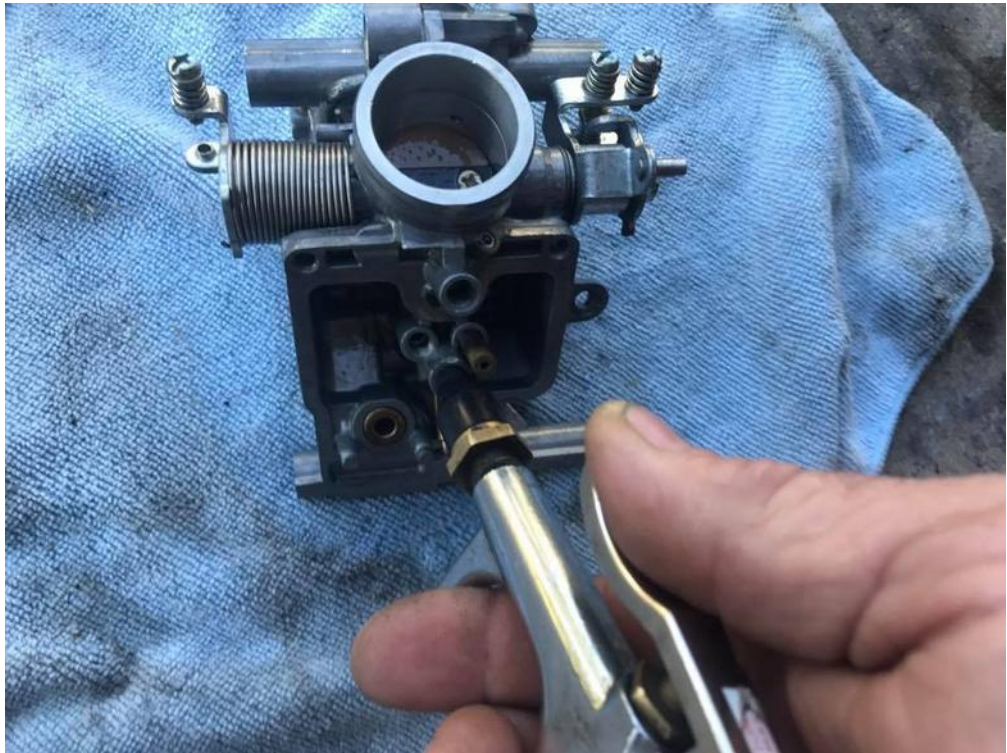
Follow up the carb spray with a good blast of air to finish it up
