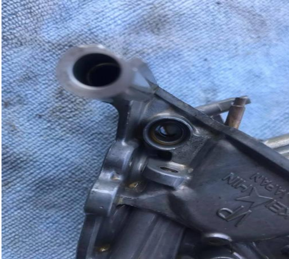
Little filters down in the fuel rail openings spray them too
