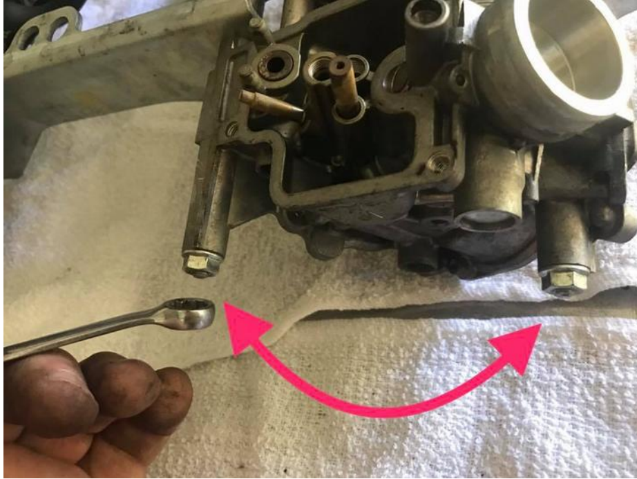
Ready to split the carbs. Remove the 2 nuts from one side of each bank
