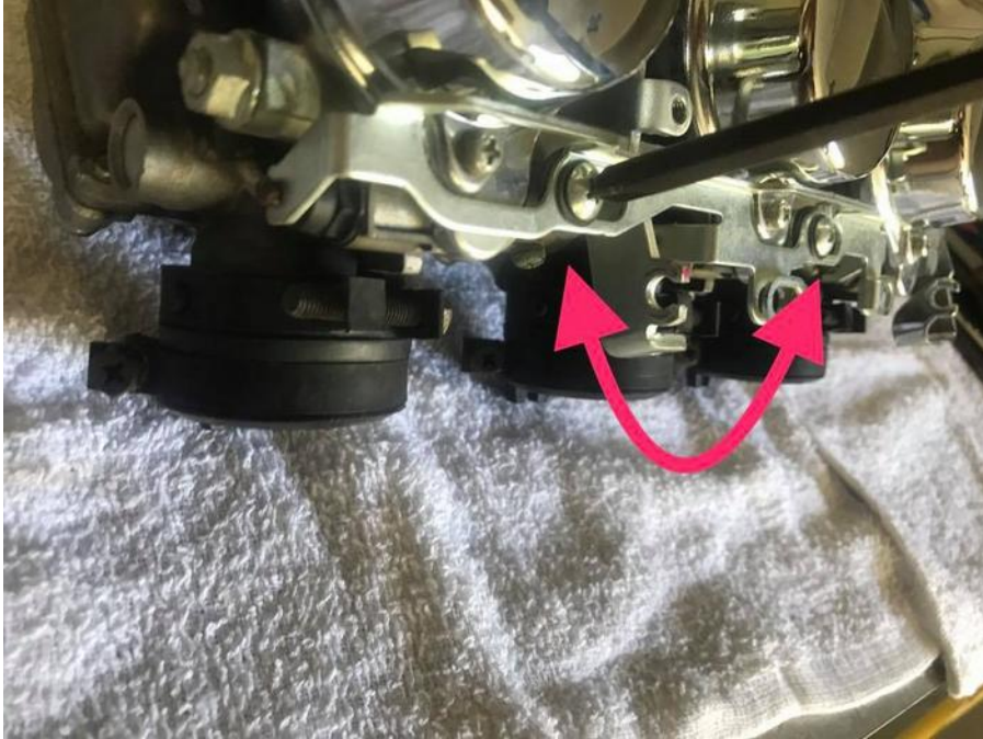
2 Phillip screws hold the choke slides on each side
