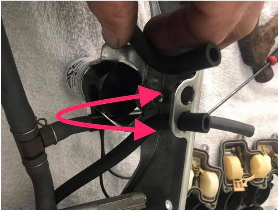
Remove the carb vent lines from the 2 holes and set them aside
