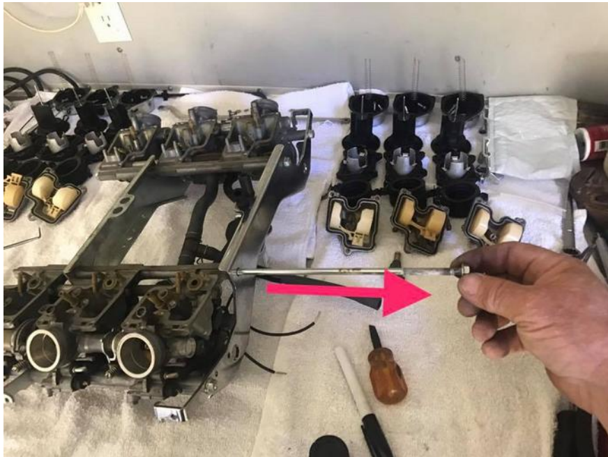
Grab the rod and slide it out. There is 4 rods to remove
