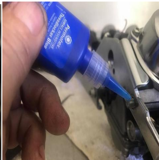
(right) I used a dab of blue loctite on the nuts. Had some come loose and lost them on one of my bikes before.
