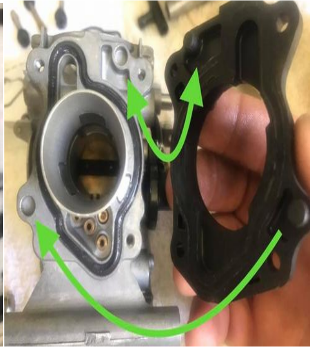
(right) Add the cover lining up the positioning tabs.
