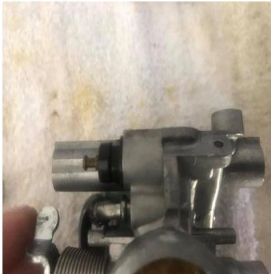
(left) Tighten with 10 mm wrench and pull out on it to make sure it moves freely.
