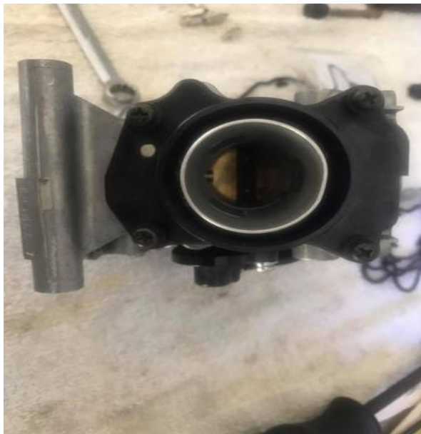
(left) Install the 4 screws and snug down
