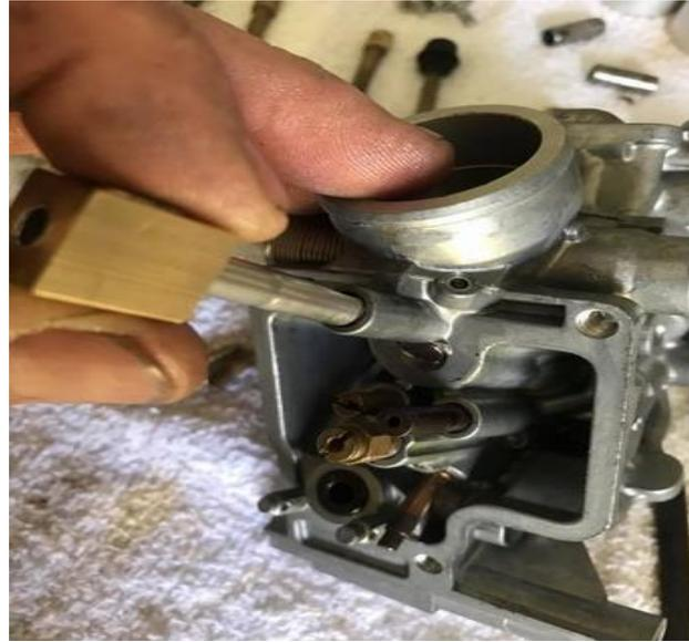
(left) Using the special tool or screwdriver if you cut slots, screw it all the way in till it just touches bottom
