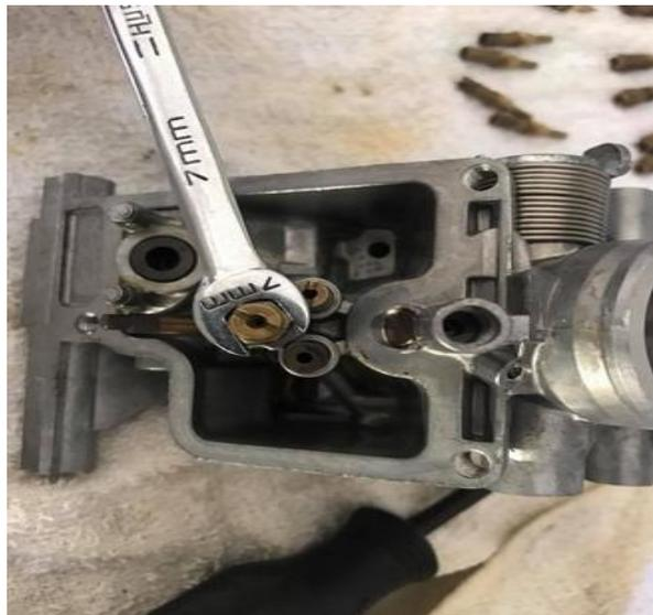
(right) Snug it down with a screwdriver or 7 mm wrench. Don't over tighten just good and snug.
