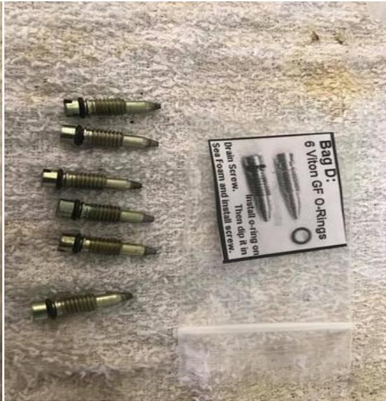
(left) 1st bag I started with was the carb drain screws. Replaced the o rings around the head
