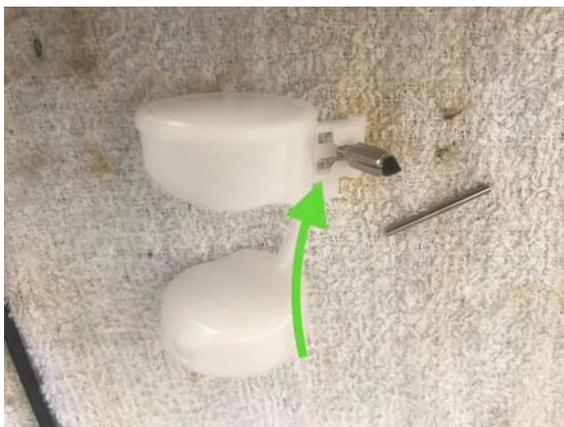
(left) Clip the needle valve into the float tab
