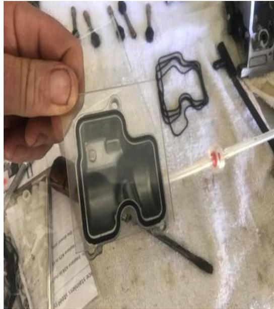
(right) Place the glass plate over the gasketed carb bowl, loosen the drain screw and apply suction to the tube, tighten the carb drain screw while pulling suction. Once the drain screw is tight you should hold vacuum in the carb bowl and hold tight to the glass plate.
