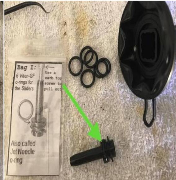
(left) It should pull right out, no need to remove the needle just replacing the o ring
