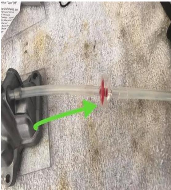
(left) Also has a neat little test tube and plate to check for leaks. Got to make sure this little red diaphragm is going the right way or you won't get any suction out of it.
