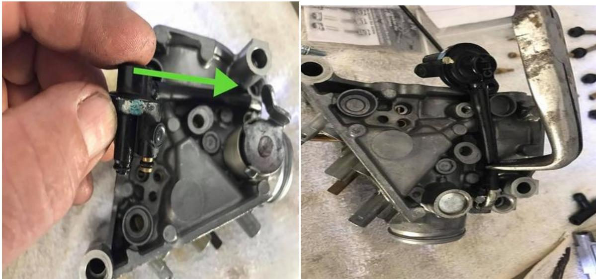
(left) I stuck a little Vaseline on the metal vacuum tube so the rubber line would slide on.
