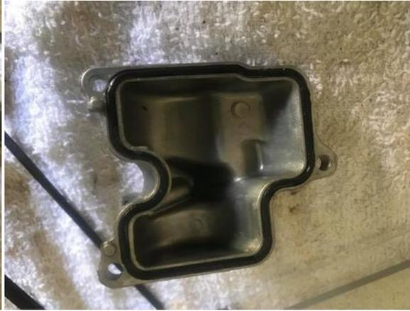
(left) After testing I added a little Vaseline to the groove for the gasket to set in and hold in place
