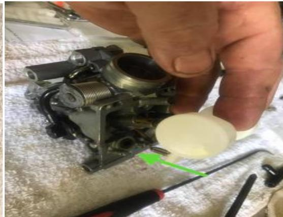
(right) Use a q tip to clean the needle valve seat in the carb body then drop the float Assembly into place with the needle valve going into the seat.
