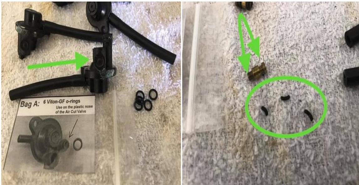
(left) New o rings replaced on air cut valves
