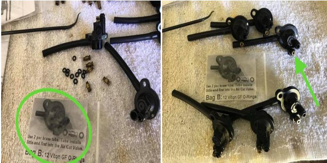
(left) Small end inserts into air cut valve first.
